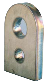
HP cut - 15mm stainless steel ArH 2 /N 2
