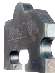
Carbon steel - 25 mm oxyfuel process
