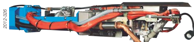
Internal welding head with single or twin wire, video and seam tracking.
