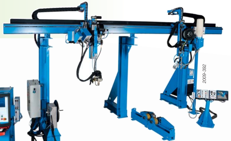
The Mechanization to customize the machine around the piece to weld.
