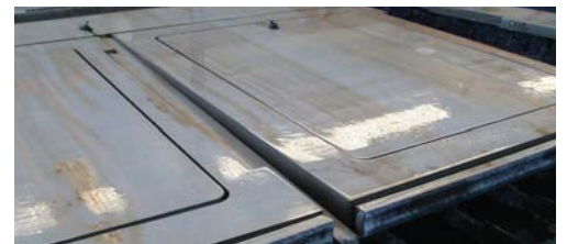
Stainless steel - water vortex - 60 mm
